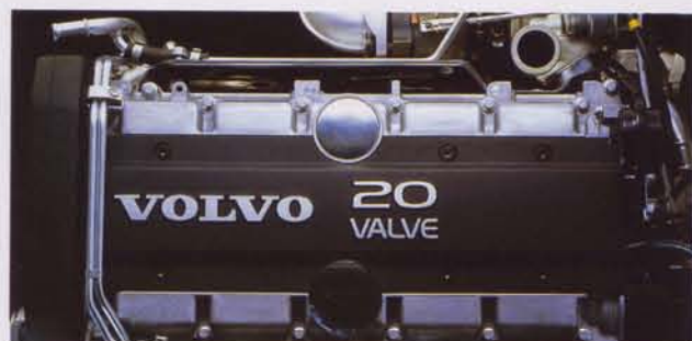
② DOHC 20 VALVE ENGINE (V70 2.5 20V)
